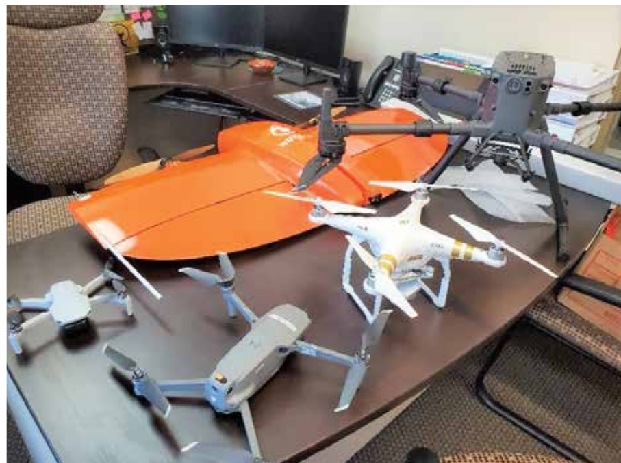
Four Rivers Drone Fleet, including: DJI Matrice 300 RTK with Zenmuse P1 camera, WingtraOne 42MP, DJI Mavic Pro 2, DJI Phantom, DJI Mini 2
